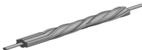
Fig. 3. Isometric view of depulping bar showing spiral and horizontal groove.
